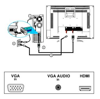
Connect the PC IN D-sub socket located at the back of the TV set to the output of PC equipment through a mini D-sub 15 pin cable (2).
